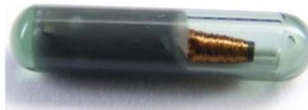
Megamos Crypto transponders are built into car keys to disable the vehicles' engine immobilisers
